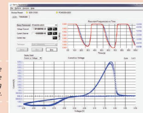
Frequency data is displayed on the potentiostat tab during acquisition. Here are both the QCM and potentiostat responses during the cycling of a Cu film on an Au electrode.
