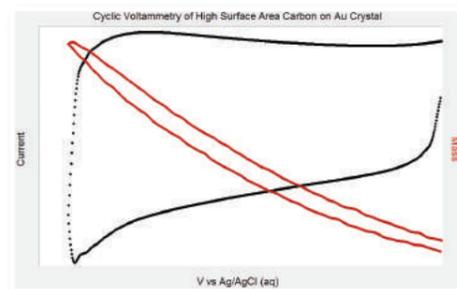
Understanding ion intercalation is an important part of battery development. Assemble your half-cell on a coated crystal and monitor mass changes as your cycle the potential – giving you insight into various charge transfer steps. Repeated cycling can allow you to understand trapping mechanisms and how they shorten device lifetime.
