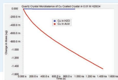
Inhibitors could be studied too – see how the mass loss rate decreases after you add an inhibitor. Or you can actively polarize your electrode using a potentiostat to induce corrosion.
