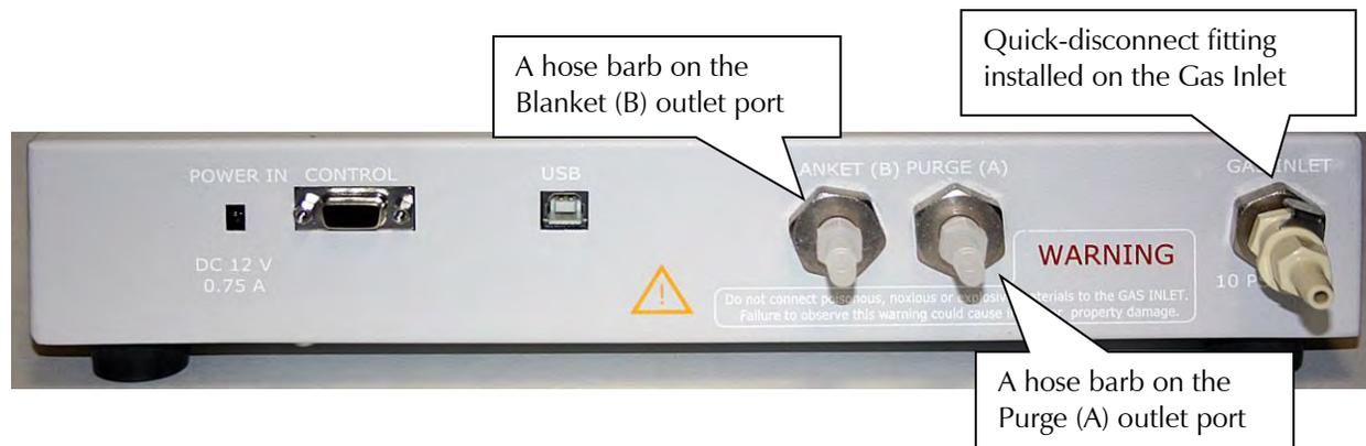
The manufacturer of the needle valve used to control gas flow rate does not recommend use of PTFE tape on any threaded fittings used in the inlet gas plumbing. Small pieces of the tape may escape into the gas flow and block the needle valve orifice. You can use PTFE thread-seal tape on the outlet ports if you desire.
