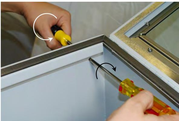
*--Disassembly of the Stir/Purge from the VistaShield*
