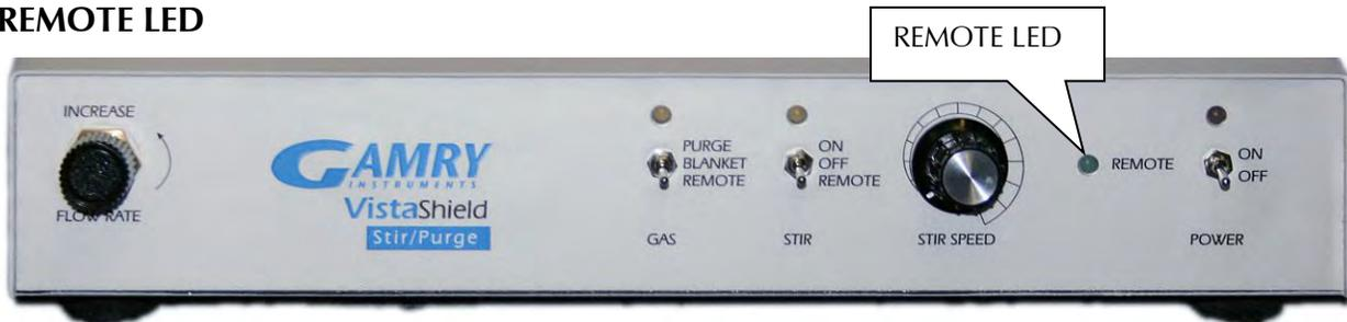
An LED is located to the left of the POWER toggle/LED. This LED is lit when one or both of the STIR or GAS switches are in the REMOTE position.
