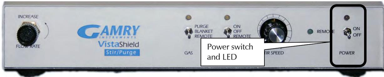
The POWER Switch and LED are located on the right of the Stir/Purge front panel. When the toggle switch is in the “ON” (up) position, the LED normally glows a steady blue.
