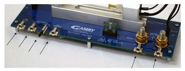
Warning: The reference banana plug is sharp and can cause injury. Be careful when connecting this pin to your cables. When it is not in use, always keep the plastic guard over the pin as a safety precaution.
