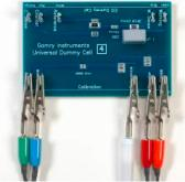
Place the dummy cell inside the Calibration Shield, close the lid, and connect the black floating-ground lead of your cell cable to the Shield's grounding post.
