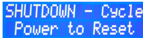
Figure 4-10 LC-display when Emergency Shutdown button is pressed
