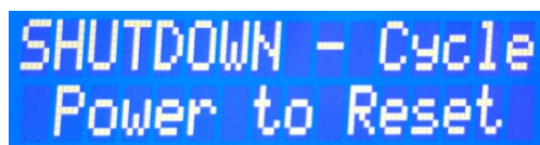
Figure 6-3 LC-display when Emergency Shutdown button is pressed
