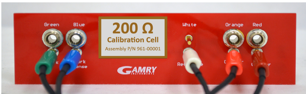
Figure 5-2 200 \Omega Calibration Cell with Leads attached for Calibration
