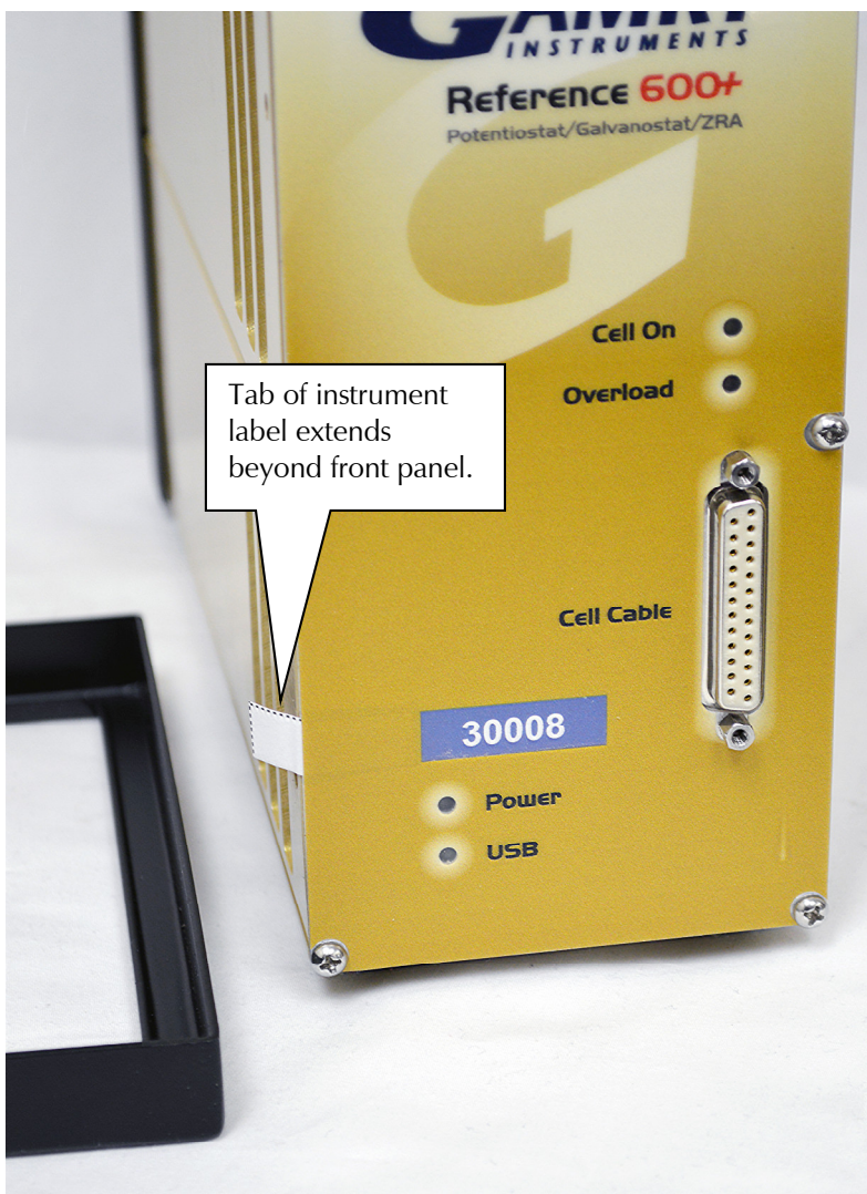
Figure 4-6 Removing the Front Bezel
