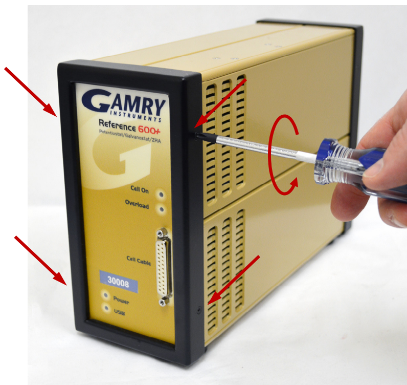
Figure 4-5 Removing the Front Bezel
