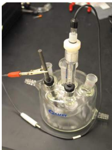
Figure 4.7: Connection of Counter and Reference Electrodes
