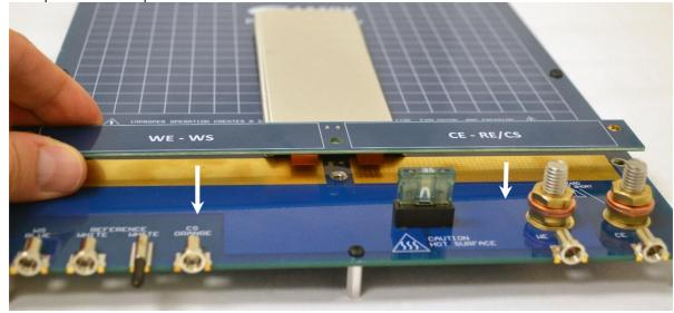
Caution: Take care not to bend or break the two metal pins during assembly. Do not bend the sense clamp too much, or it will break.
