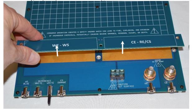
**Caution:** The underside of the sense clamp has two metal pins. These are used for four-point measurements. Take care not to bend or break them during assembly.
