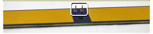
3. Place the pouch cell on the printed-circuit board, sliding the positive electrode over the left (Working) and the negative electrode over the right (Counter) pads. Lower the sense clamp onto the board. Be careful to line up the two small pins with the holes in the board.
