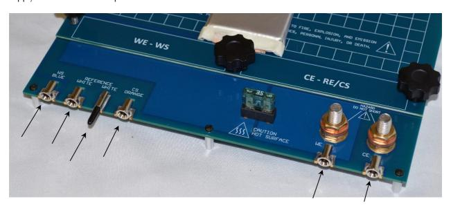
Warning: The reference banana plug is sharp and can cause injury. Be careful when connecting this pin to your cables. When it is not in use, always keep the plastic guard over the pin as a safety precaution.
