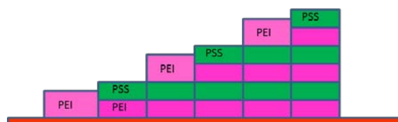
Figure 3. Model for the build up of the PEI/PSS polymer multilayer.
