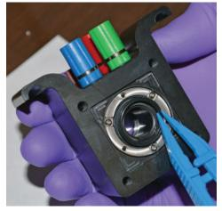
Place the three goldplated, spring-loaded contact pins into the three empty holes in the metal ring. The smaller, springloaded ends must be upward, away from the cell body.
