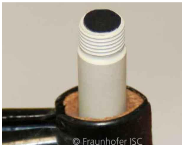
Fig. 5. Large electrode holder with foil electrode placed on top.
