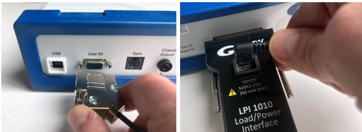
Figure 4-4 Installation of the LPI Power Cable at the rear of an Interface 1010 potentiostat (left) and micro USB connector of the LPI1010 D-sub Module (right)
