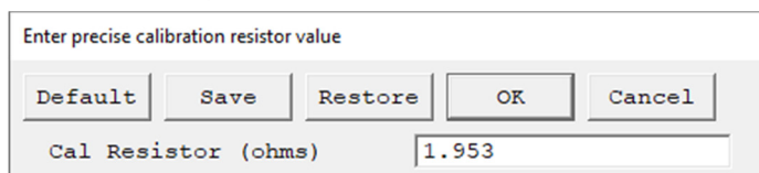
Figure 5-8 Entering Resistor value of the Calibration Cell
