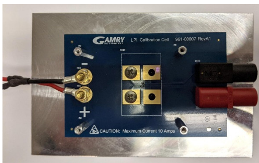
Figure 5-7 LPI1010 200 mΩ Calibration Cell with connected cell leads
