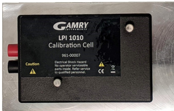
Figure 5-3 LPI1010 200 m \Omega Calibration Cell with cover
