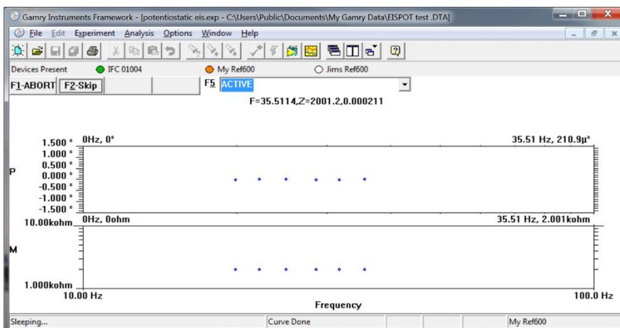
The Interface 1000 (IFC 01004) in this system is shown with a green indicator because it is installed and ready to run. The Reference 600 labeled My Ref600 has an orange indicator because it is recording the EIS spectrum shown on the screen. The Reference 600 labeled Jims Ref600 has a white indicator, showing it is plugged in but cannot be used. This is an indication of a version mismatch between Gamry Instruments Framework software and the instrument's firmware.
