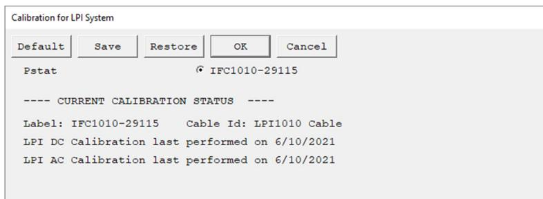
The setup window shows the potentiostat used for calibration. Select the correct device for the LPI calibration. Further below in the setup window are the previous LPI calibration results listed including the date. If a calibration was not successful, an error message is shown instead.
