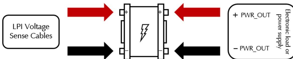
Connect the free ends of the LPI Voltage Sense Cables to the DUT. If the DUT does not connect directly to the male banana plugs on the LPI Voltage Sense Cables, use an adapter appropriately rated for the voltage of the DUT. The red cable connects to the positive (+) contact, the black cable connects to the negative (-) contact of the DUT.
