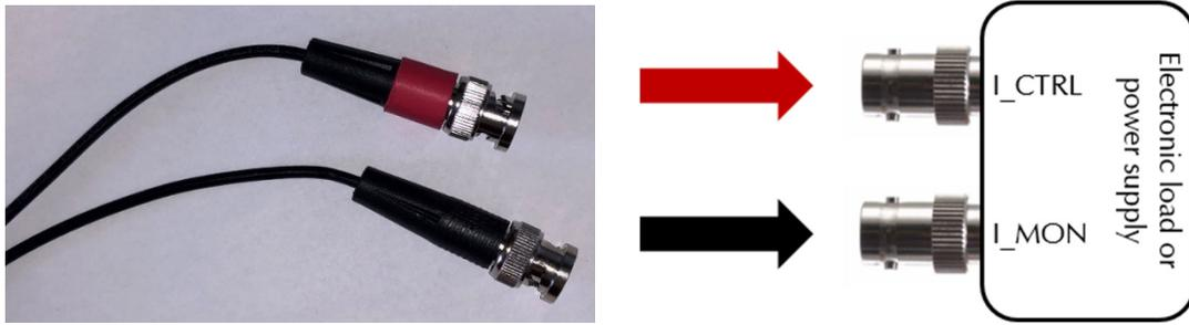
The red-marked BNC connector lead is the current control (I\_CTRL) output of the LPI1010 and goes to the mating current control input of the electronic load or programmable power supply. The black-marked BNC connector lead serves as current monitor (I\_MON) of the LPI1010 and connects to the current monitor output of the electronic load or programmable power supply.
