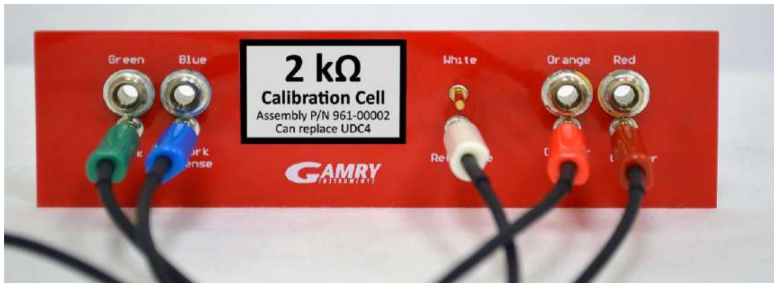
Figure 3-4 2 kΩ Calibration Cell with Leads Attached for Calibration
