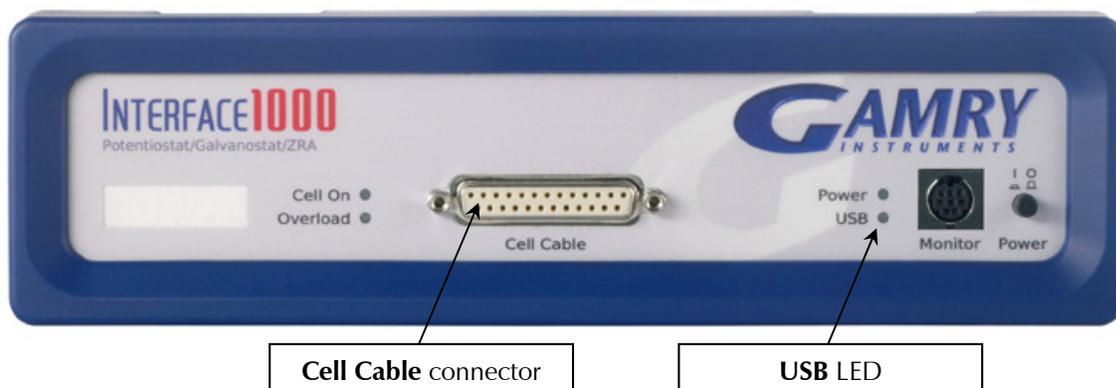
All Gamry standard cell cables have a 25-pin D-connector on one end and a number of leads terminated with banana plugs on the other. The D-connector end of the cable is connected to the **Cell Cable** port on the front of the Interface 1000. Always use the knurled screws on this cable to hold the cable in place.
