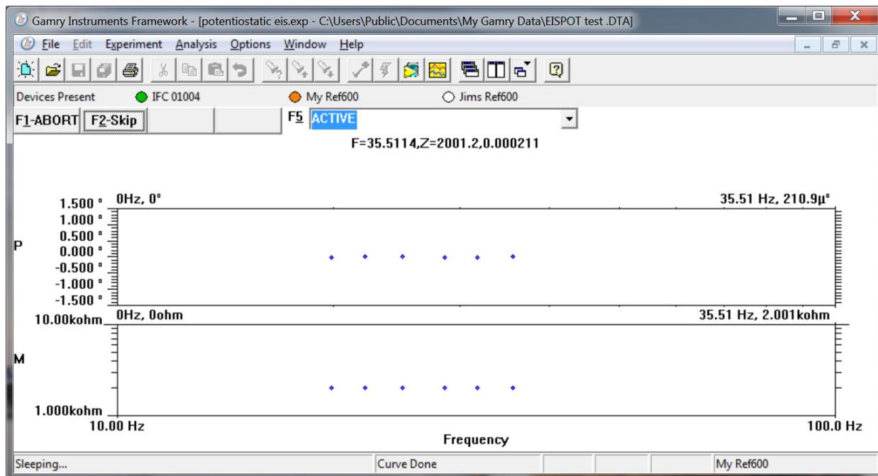
The Interface 1000 (IFC 01004) in this system is shown with a green indicator because it is installed and ready to run. The Reference 600 labeled My Ref600 has a red indicator because it is recording the EIS spectrum shown on the screen. The Reference 600 labeled Jims Ref600 has a white indicator, showing it is plugged in but cannot be used. This is an indication of a version mismatch between firmware and instrument.
