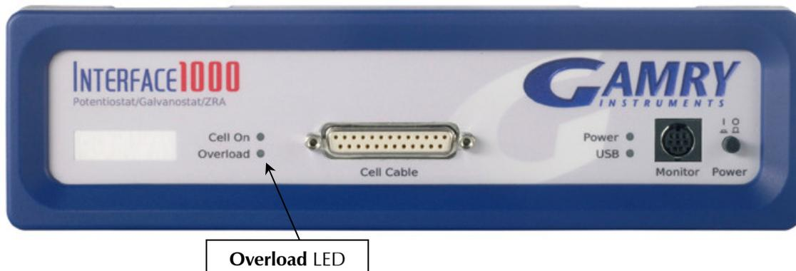
The **Overload** LED is normally unlit. When it glows red, some circuit in the Interface 1000 has exceeded its normal operating limit. Conditions that generate Overloads include:
