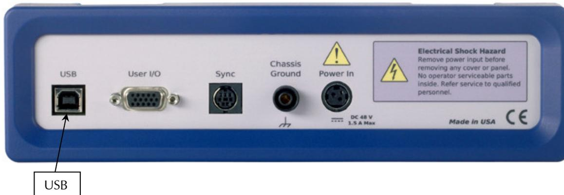
The USB connection can be “hot-plugged.” This means both the computer and the Interface 1000 can be powered-up before the USB cable is plugged in. Unlike many other instrument system connections, you need not power down the system before plugging in the USB.
