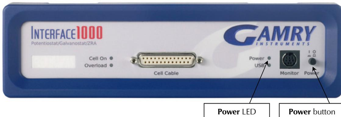
Watch the **Power** LED as the Interface 1000 powers up. It flashes slowly four or five times (depending on the amount of software loading), then glows a steady blue. This process could take as long as 15 seconds. The Interface 1000 fan runs at low speed once the **Power** light stops flashing. If you do not see four or five blinks and then a steady blue color, see Appendix D for a table of blink codes.
