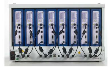
Connect the power cord from the wall outlet (mains) to the IPH. Connect USB cable from the **HOST** USB connector on the back of the IPH to your host computer.
