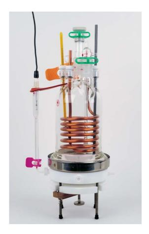
The Gamry Instruments Flexcell<sup>TM</sup> is a versatile electrochemical cell designed to counteract a problem that plagues most cells crevice corrosion around the specimen seal. First popularized by Avesta Steel, the cell utilizes a flooded gasket seal design to inhibit crevice corrosion between the sample and its holder. This simple yet elegant design results in an easy to use, reliable, crevicefree system.
