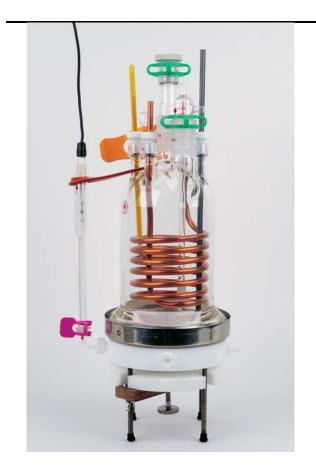
The Gamry Instruments Flexcell<sup>™</sup> is a versatile electrochemical cell designed to counteract a problem that plagues most cells -- crevice corrosion around the specimen seal. First popularized by Avesta Steel, the cell utilizes a flooded gasket seal design to inhibit crevice corrosion between the sample and its holder. This simple yet elegant design results in an easy to use, reliable, crevice-free system.
