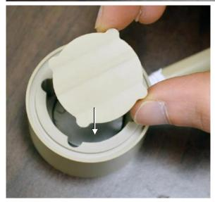
15. Screw the compression plate into the cell body, so that it is tight, and as far as it can go, so that the sample contacts the pins reliably.
