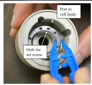
9. Feed the wire through the port and small hole, and screw the rod into the cell body. The metal ring may twist while you do this, so hold the metal ring with the tweezers in two holes.
