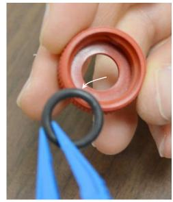
3. Add the new O-ring (with a slightly smaller inner diameter of 9.5 mm, that comes with the Flat Sample Holder) into the cap.
