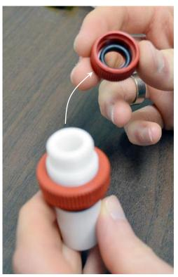
2. Remove the existing O-ring from the cap.
