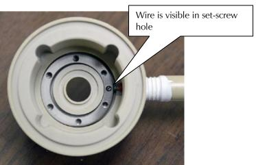
10. Thread the M2.5 set screw into its receptacle, and tighten with the small screwdriver until the top of the set screw is recessed below the metal ring.
