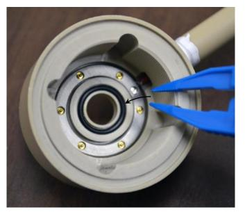
13. Place your sample electrode metal into the cell body. Its diameter may be between 2.5 and 3 cm; its maximum thickness is 7 mm.
