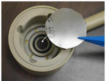
14. Drop the stopper plate into the cell body on top of your sample. Line up the tabs with the recesses in the cell body.
