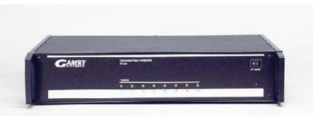
The Gamry ECM8 Electrochemical Multiplexer is designed for electrochemical applications. The ECM8 Multiplexer connects up to eight electrochemical cells to one Gamry Potentiostat/Galvanostat/ZRA. This converts a single Potentiostat into a powerful instrument capable of automated sequential electrochemical experiments. Applications for the ECM8 include corrosion inhibitor testing, EIS
