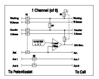
In addition, each channel of the ECM8 Multiplexer has an optional Auxiliary A/D Switch that can connect any one of eight connectors to one common point for additional experimental versatility.
