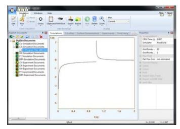
**CA simulation and concentration profiles** ChronoAmperometry and concentration profiles can also be simulated with any of the systems described in the CV section
