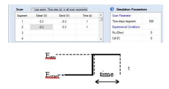
**CA** setup and anatomy of the CA signal Three parameters define the signal.  $E_{start}$ ,  $E_{end}$ and time are available on the setup screen as shown.
