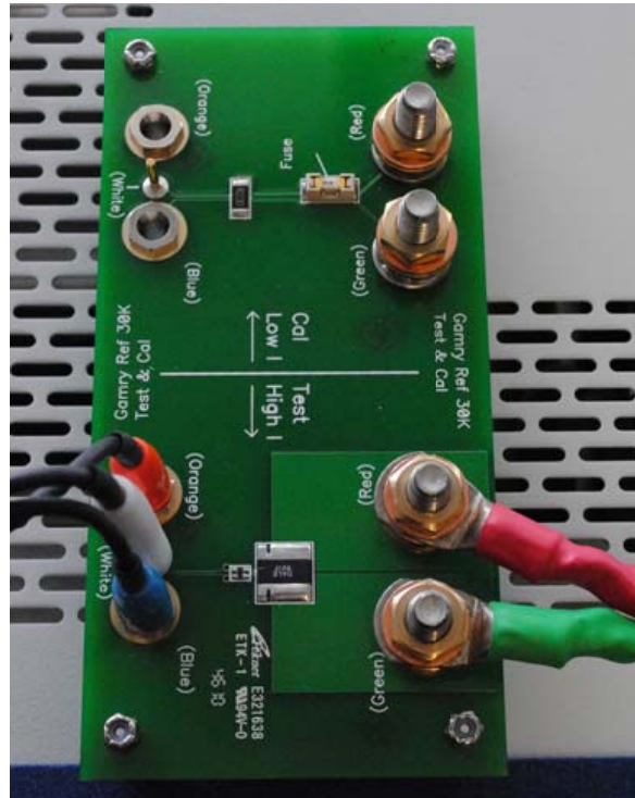
Figure 3-3 Connections to the Test Side of the Test and Cal Fixture
