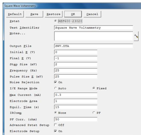
Typical setup window in the Gamry Framework. Setting the parameters for an electrochemical experiment in the Framework is easy—just fill in the fields! Click **Notes** to add specific information to the data file about your sample. Save data in the **Output File**. The text boxes “remember” the last entered value, accelerating parameter entry. Click **Default** to re-enter the default values. **Save** a setup and **Restore** it later. Click **OK** to run the experiment.
