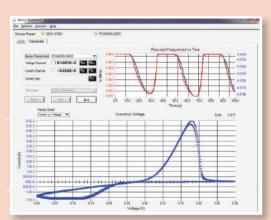
Frequency data is displayed on the potentiostat tab during acquisition. Here are both the QCM and potentiostat responses during the cycling of a Cu film on an Au electrode.
