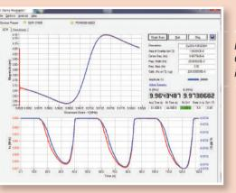
Data acquisition is controlled with one program. QCM control is on one tab while potentiostat control is on another tab.
