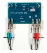
Place the UDC4 inside the Gamry Calibration Shield, close the lid, and connect the black floating-ground lead of your cell cable to the Shield's grounding post.
