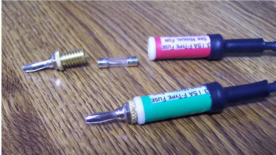
Figure 5-1 Open Fuse-holder Showing Fuse
