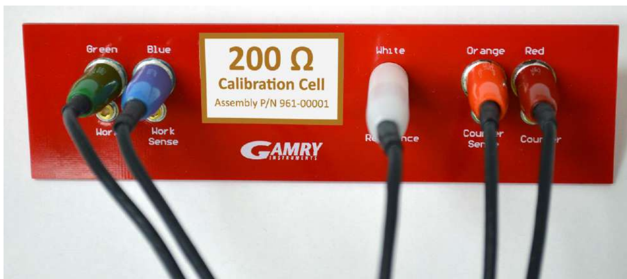
Figure 4-1 Interface 5000 Calibration Cell with Leads Attached for Calibration
