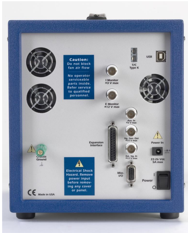
Figure 3 - 2 Rear Panel of the Reference 3000
