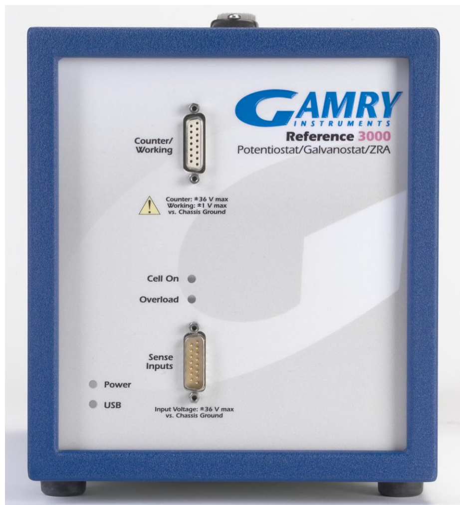
Figure 3 - 1 Front View of a Reference 3000 without AE Option
