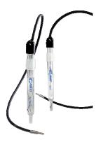
The impedance of your Reference Electrode should be less than 1 kohm. An impedance higher than 1 kohm is not good and an impedance higher than 5 kohm is unacceptable and must be corrected. With a Gamry Reference Electrode, the problem is easily corrected by changing the Vycor Frit.
